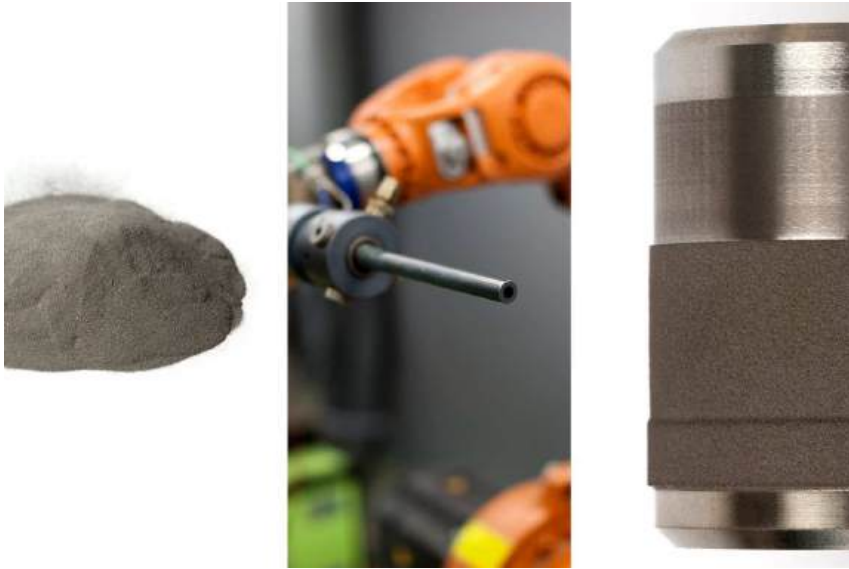
Figure 20.4 Refining of steel parts using thermal spraying processes by Putzier. Photo: Jens Putzier.
