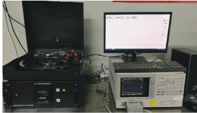
Figure 9. The junction capacitance parameter test platform for diodes.
