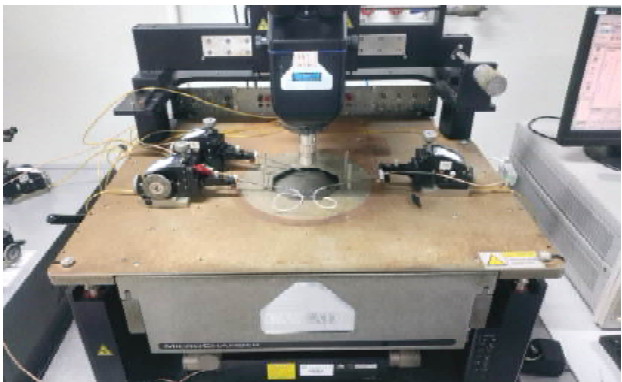
Figure 5. The I-V static parameter test layout of the 2CZ106C.
