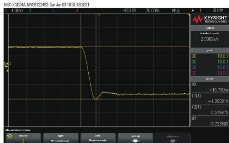
Figure 14. The reverse recovery waveform of 2CZ109C diode.
