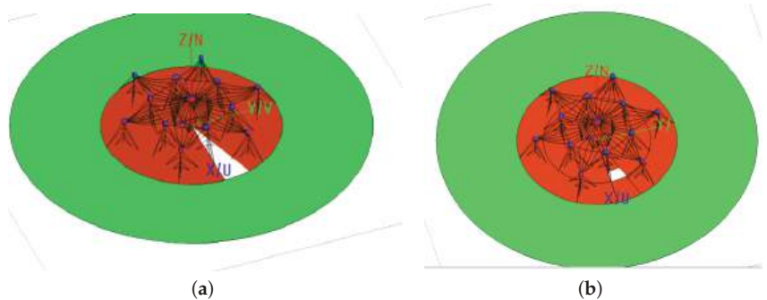
Figure 6. Schematic diagram of the second type model; the darkly colored area is the functional part of the ground network, the lightly colored area is the non-ideal ground, and the blank area is the fracture in the ground network: (a) The first model. (b) The second model.
