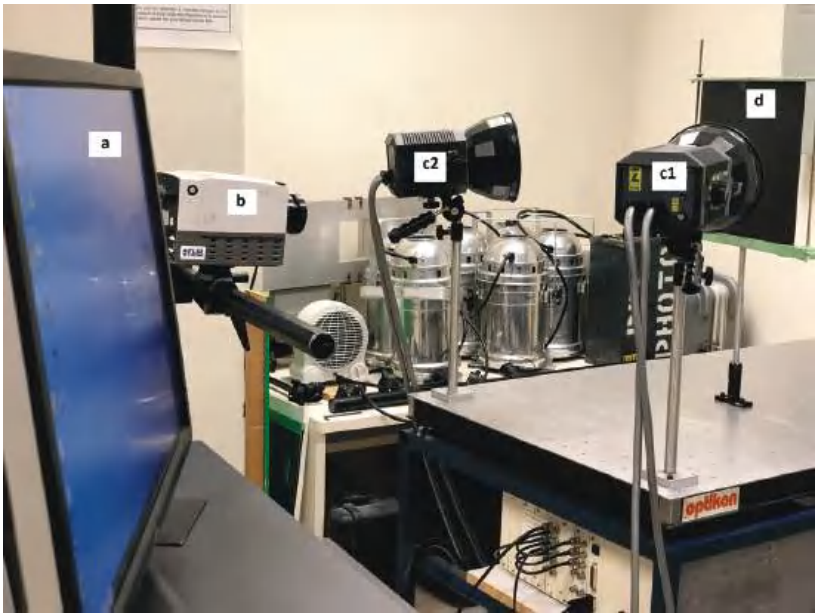
Figure 2. (a) CTA CFRP plate, where Z is the defect depth, and labels are used to identify the location of each defect; (b) pulsed thermography setup. a, PC; b, IR camera; c1 and c2, left and right flashes; d, CFRP specimen.
