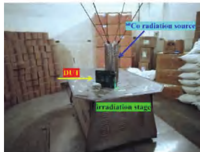
Figure 2. DUT in the terminal of the ^{60}\text{Co} irradiation.
