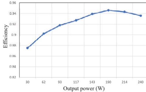
**Figure 12.** Measured efficiency of the proposed converter.
