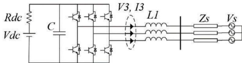
Figure 4. The VSC for unbalanced condition illustration.
