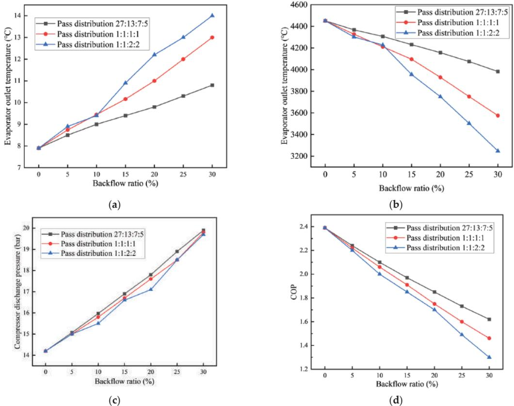
**Figure 8.** Influences of the backflow rate on air conditioning performances under different ambient temperatures. (a) Evaporator exit temperature; (b) evaporator heat rejection; (c) discharge pressure; and (d) COP.
