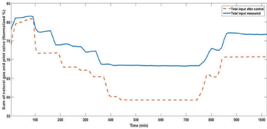
**Figure 16.** Total fuel input to the plant (pilot valve flow + NG flow) showing significant reduction in fuel or natural gas consumption (dashed orange) if operated totally on NG (i.e., premix mode) over the existing operation fuel consumption (blue).
