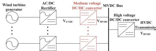
Figure 2. HVDC transmission system with MVDC grid.
