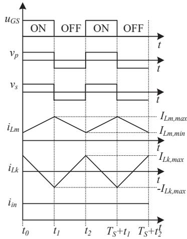
Figure 4. Theoretical waveforms of the proposed converter.
