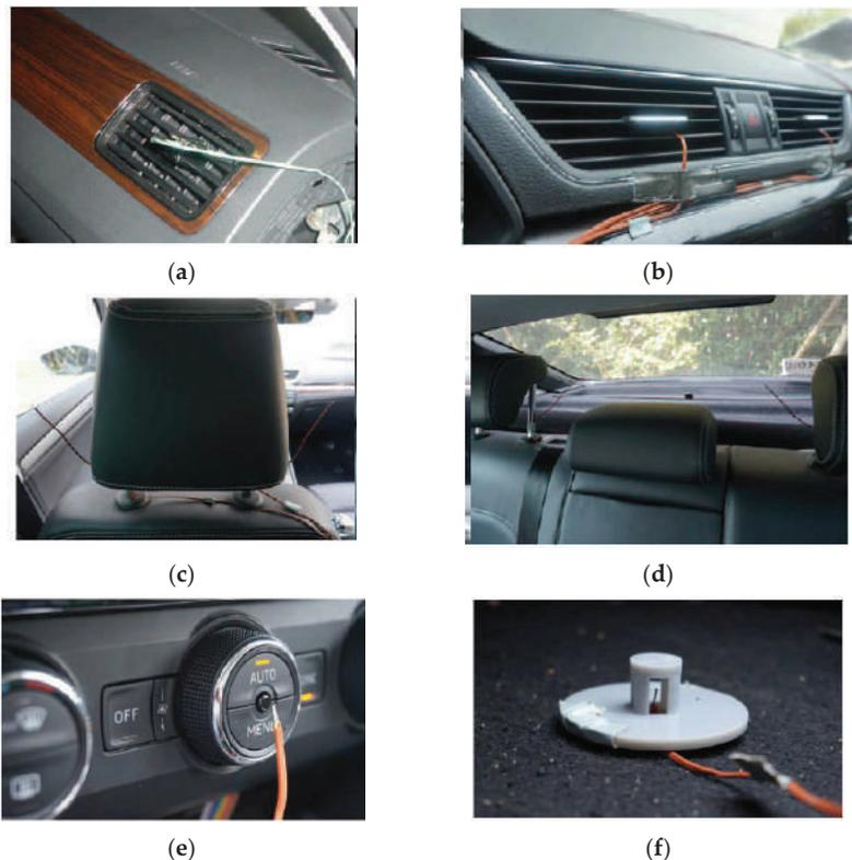
**Figure 4.** The measurement points of temperature sensor in the cabin. (a) Side air outlet; (b) Middle air outlet; (c) Front seat passenger; (d) Rear seat passenger; (e) Dashboard area; (f) Cabin bottom.
