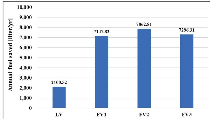
**Figure 10.** Annual fuel saving on the model vehicles platooning compared to the single moving vehicle (SV) at a 0.5 L gap.
