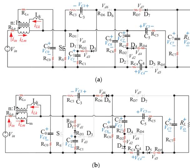
Figure 8. The equivalent circuits considering all the non-idealities: (a) Mode 1; (b) Mode 2.
