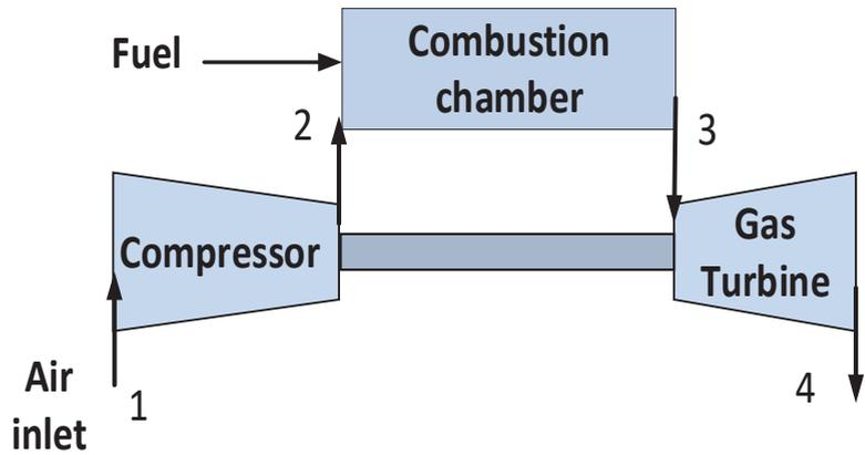
Figure 1. Main components of gas turbine unit [3].
