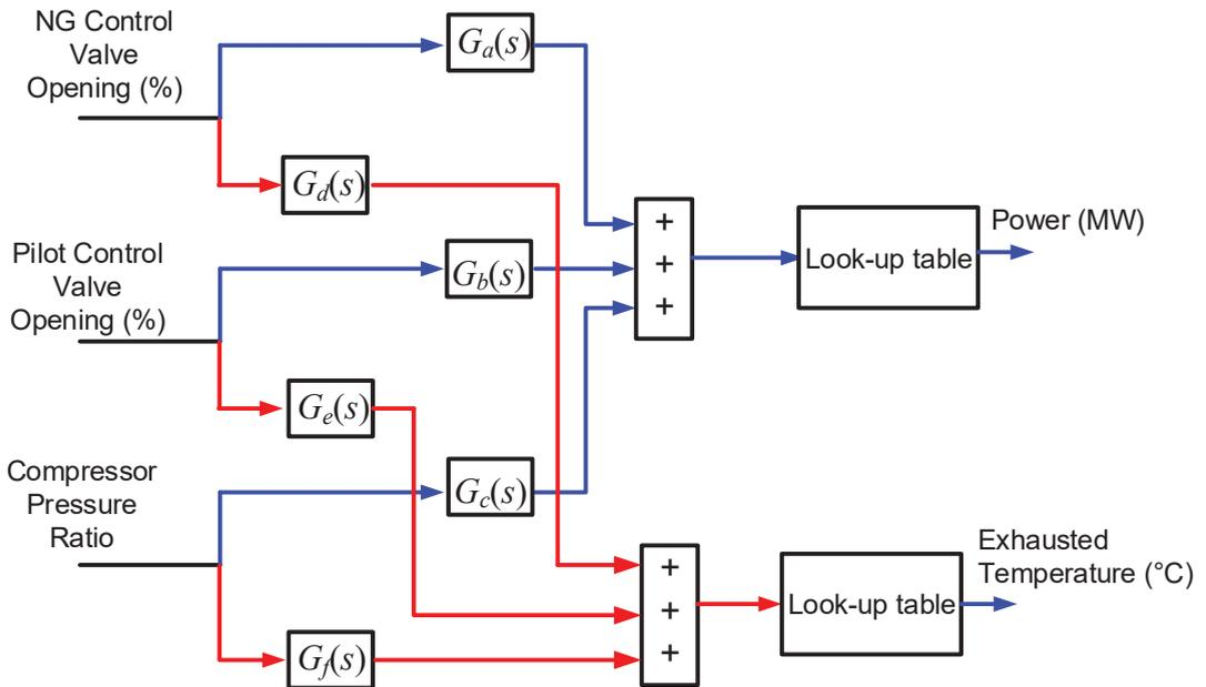
**Figure 5.** The Mathematical Model of the Gas Turbine, Red: the input signal flows through the system to the exhausted temperature, Blue: the input signal flows through the system to the output power.
