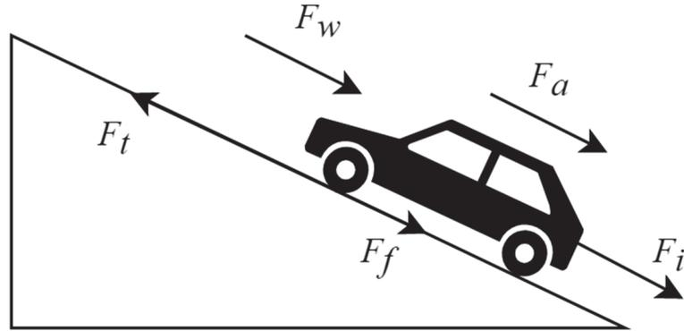
**Figure 2.** Diagram of electric vehicle longitudinal dynamics.
