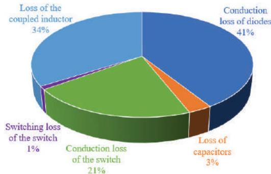
**Figure 9.** Loss distribution of the proposed converter.
