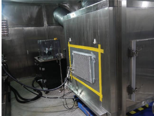
**Figure 5.** The heat exchanger performance test platform.
