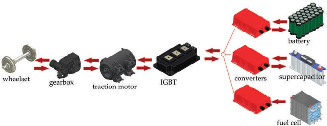
Figure 1. Power flow according to traction system topology.
