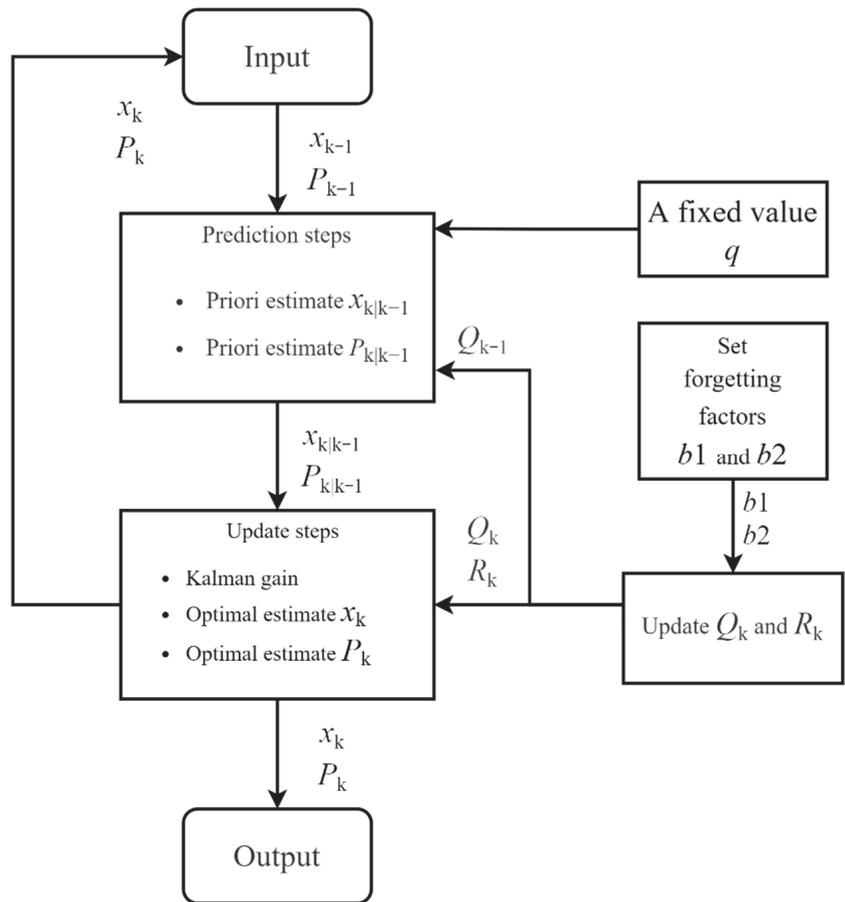
**Figure 4.** Flow chart of improved adaptive Kalman filter.
