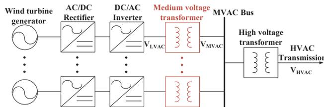
Figure 1. HVAC transmission system with MVAC grid.
