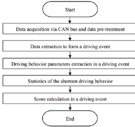
Figure 17. The evaluation flow chart of driving behaviour.
