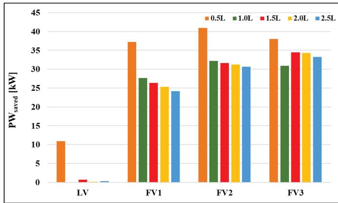
**Figure 9.** Tractive power ( $PW_{\text{saved}}$ ) saved on the vehicles platooning compared to SV at 100 km/h.
