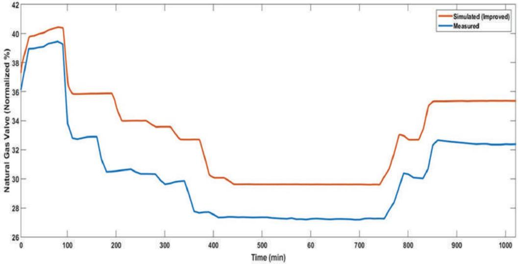
**Figure 14.** The Pilot valve dynamics, showing the existing and actual fuel oil (diffusion mode)/natural gas (premix mode) consumption (blue) and the simulated (improved dynamics (orange)). Notice: higher fuel consumption from the Pilot valve.
