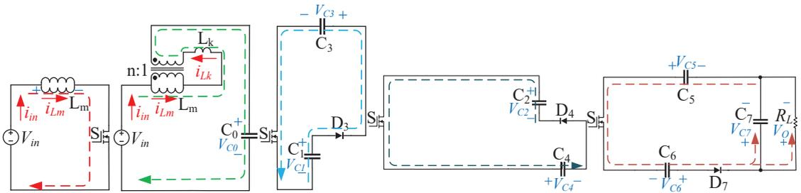
Figure 6. Simplified equivalent circuits of Mode 1.
