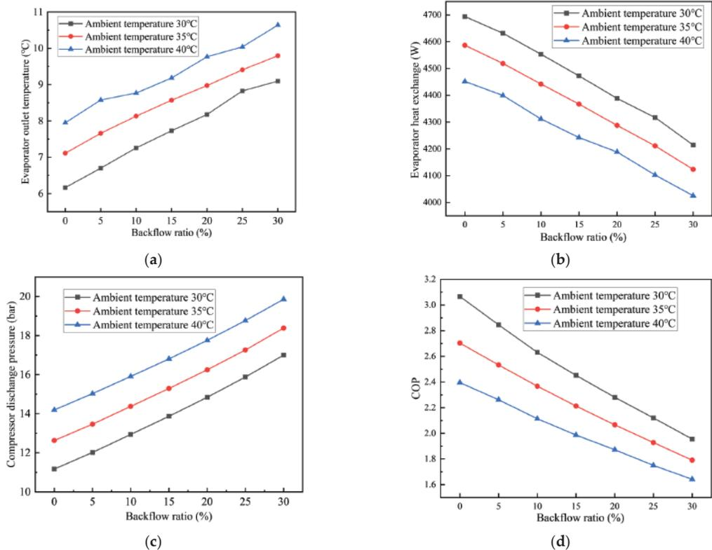
**Figure 7.** Influences of backflow rate on air conditioning performances under different ambient temperatures. (a) Evaporator outlet temperature; (b) evaporator heat rejection; (c) compressor discharge pressure; and (d) COP.
