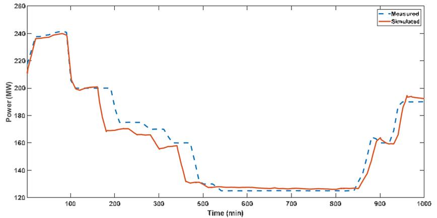
Figure 9. Measured and simulated output power responses.
