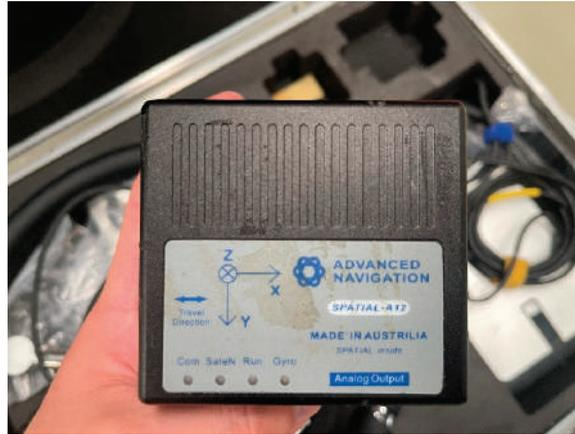
**Figure 5.** IMU of high accuracy.
