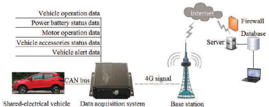
**Figure 2.** The acquisition process of the NDS data.
