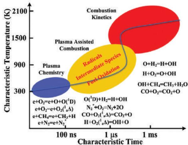
Figure 11. Schematic of timescales for PAC kinetics [61].
