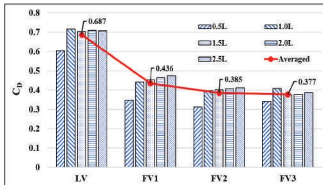
**Figure 4.** Variation in drag coefficient (C<sub>D</sub>) of each model vehicle in platooning with the change in the gap.
