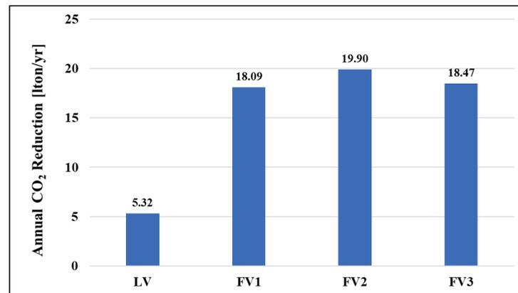
**Figure 11.** Annual CO<sub>2</sub> reduction in platooning vehicle driving compared to the single moving vehicle (SV) at a 0.5 L gap.
