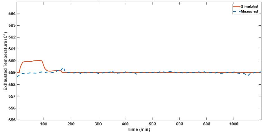
Figure 10. Measured and simulated exhausted temperature responses.
