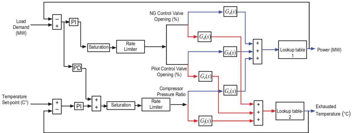
Figure 11. Simulink model with the suggested controller.
