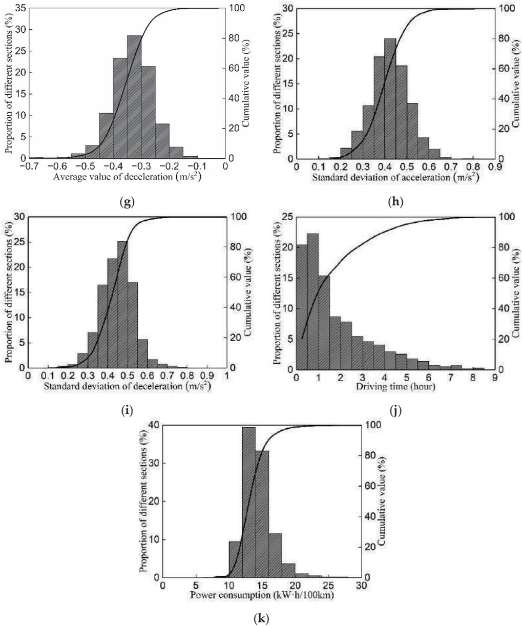
**Figure 16.** The distribution of different indexes: (a) The number of rapid accelerations per 100 km; (b) The number of sudden brakings per 100 km; (c) The number of rapid turns per 100 km; (d) The number of speeding occurrences during steering per 100 km; (e) Standard deviation of vehicle speed; (f) Average value of acceleration; (g) Standard deviation of acceleration; (h) Average value of deceleration; (i) Standard deviation of deceleration; (j) Driving time per trip; (k) Power consumption.
