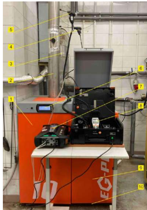
Figure 2. Boiler test stand: 1—test boiler, 2—chimney, 3—Pitot tube, 4—fume probe, 5—flow probe, 6—boiler controller, 7—Testo 350—flow meter, 8—Testo 380—PM meter, 9—pellet reservoir, 10—scales.
