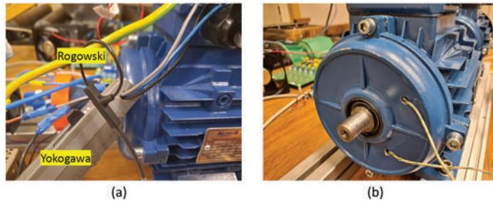
**Figure 8.** (a) Yokogawa Hall-effect and PEM Rogowski sensors. Both provide 50 MHz bandwidth and a maximum current of 30 A; (b) end-frame with the cables connected to two temperature sensors. Temperature sensors are attached to the end coils.
