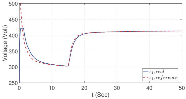
Figure 7. AES voltage control during regenerative braking.
