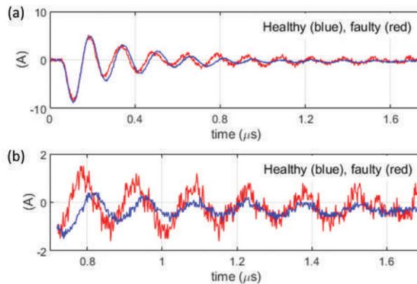
**Figure 12.** (a) Transient common mode current for the healthy and faulty cases. (b) Windowed common mode current  $i_{0W}$ ; obtained by applying a window  $W$  to  $i_0$ .  $W = 1$  for  $0.75 \mu\text{s} < t < 1.7 \mu\text{s}$ ;  $W = 0$  otherwise.
