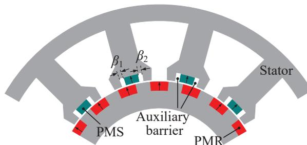
Figure 13. Schematic diagram of the stator with AB.
