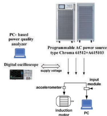
Figure 2. Simplified diagram of the measurement setup.
