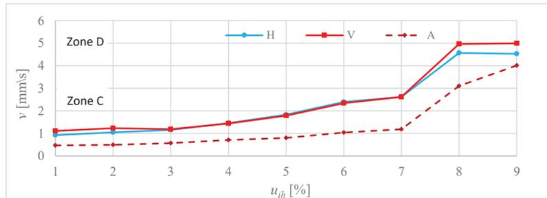
**Figure 11.** Measured broad-band vibration velocity in the horizontal (H), vertical (V), and axial (A) directions versus the voltage interharmonic value  $u_{ih}$  for motor2 and interharmonic frequency  $f_{ih} = 101$  Hz.
