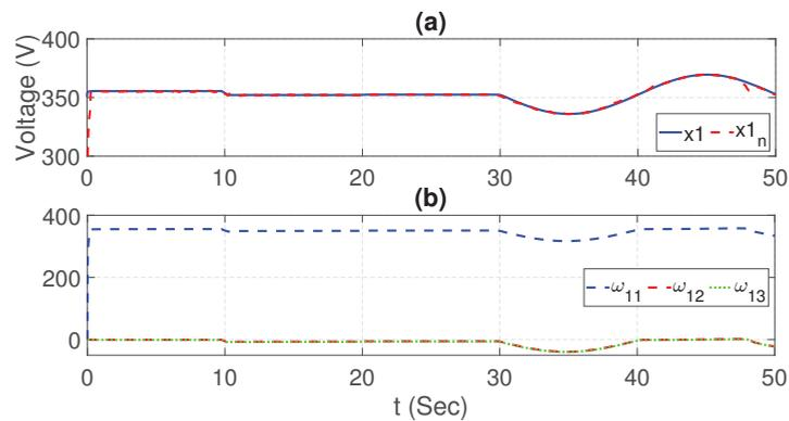
**Figure 1.** Voltage identification (a) and NN’s weights (b).
