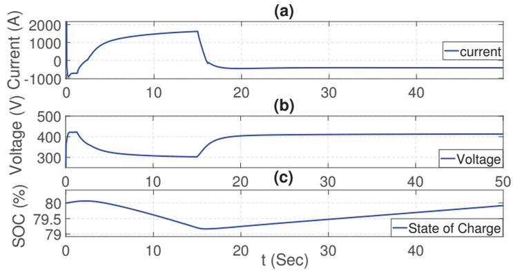
**Figure 9.** AES supercapacitor SOC. (a) Illustrate the obtained current during the vehicle operation, (b) the obtained voltage during the vehicle operation and (c) the state of charge of the supercapacitor during the operation.
