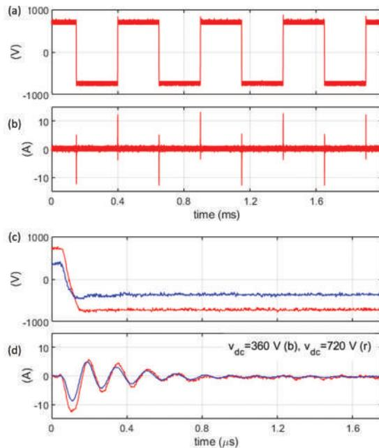
Figure 5. (a) Common mode voltage; (b) common mode current. FB switches at 2 kHz,  $v_{dc} = 720$  V; (c,d) zoomed signals for the case of  $v_{dc} = 720$  V (red) and  $v_{dc} = 360$  V (blue), respectively.
