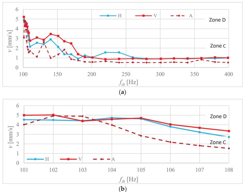
**Figure 10.** Measured broad-band vibration velocity in the horizontal (H), vertical (V), and axial (A) directions versus the voltage interharmonic frequency for motor2 and interharmonic value  $u_{ih} = 9\%$ . Figure (b) is an enlarged fragment of Figure (a).
