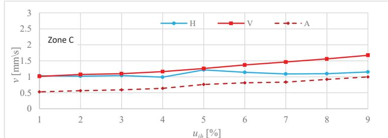
**Figure 12.** Measured broad-band vibration velocity in the horizontal (H), vertical (V), and axial (A) directions versus the voltage interharmonic value  $u_{ih}$  for motor2 and interharmonic frequency  $f_{ih} = 175$  Hz.
