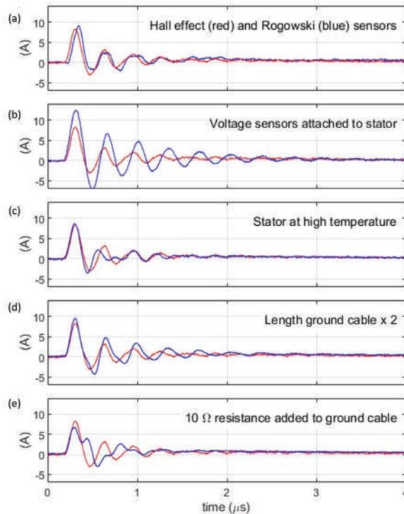
**Figure 9.** Measured common mode current: (a) Hall sensor vs. Rogowski coil at ambient temperature; (b) effect of a voltage sensor attached to the stator; (c) effect due to temperature; (d) effect due to ground cable length; (e) effect due to ground cable resistance.  $V_{dc} = 360$  V. Hall sensor was used for cases (b–e). The trace in red in (a) is shown in all the subplots for reference.
