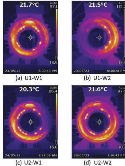
**Figure 11.** Captures of the thermal imaging camera after test #28 when the stator is fed from a *dc* voltage source between terminals indicated in the subcaptions. The stator has 24 slots, single-layer winding.
