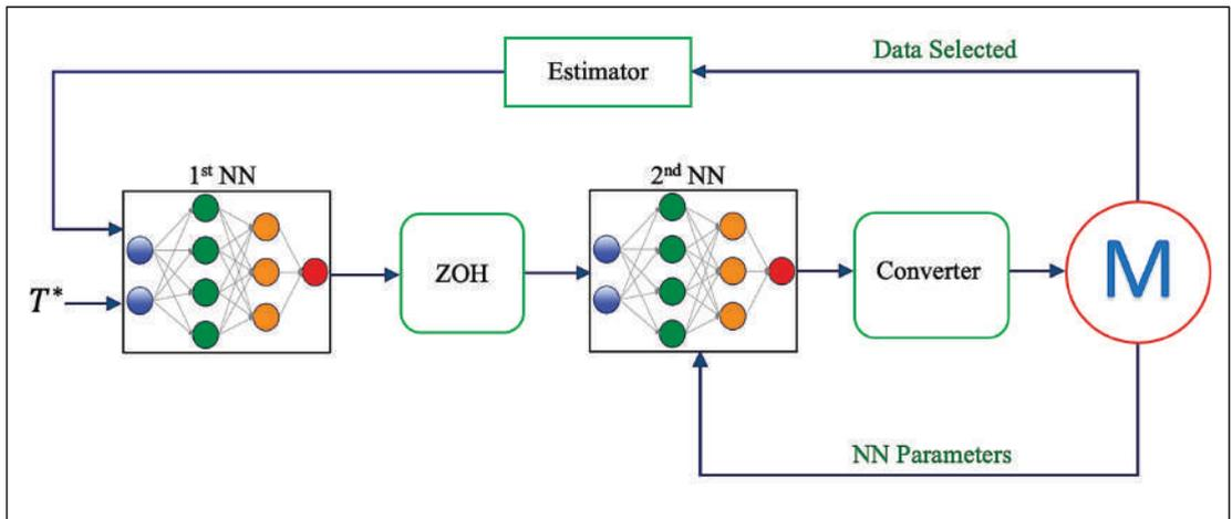
**Figure 1.** The proposed framework for minimizing torque ripples.
