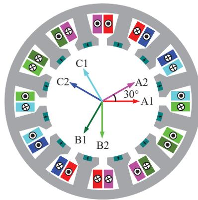
Figure 18. The DPMV with DTP-30° winding configuration.
