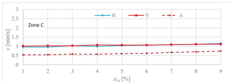
**Figure 13.** Measured broad-band vibration velocity in the horizontal (H), vertical (V), and axial (A) directions versus the voltage interharmonic value  $u_{ih}$  for motor2 and interharmonic frequency  $f_{ih} = 208.3$  Hz.
