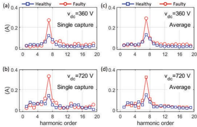
**Figure 14.**  $|FFT(i_{0W})|$  [see Figure 12b]. Left (a,b): single capture, right (c,d): average of eight successive captures. Top (a,c):  $V_{dc} = 360$  V, bottom (b,d):  $V_{dc} = 720$  V. Blue/Red: healthy/faulty machine.
