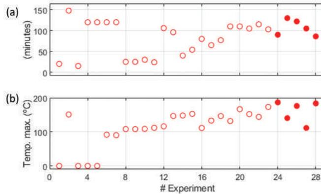
**Figure 7.** Summary of experiments: (a) length in minutes; (b) maximum temperature. Experiments marked with a solid dot indicate that a decrease in phase-to-phase insulation had been detected with the insulation tester.
