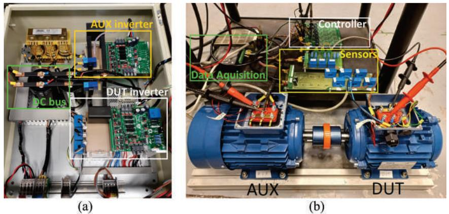
**Figure 3.** Test bench pictures: (a) back-to-back inverters and, (b) DUT and AUX motors. Rated values:  $V = 440 \text{ V}$ ;  $I = 2.74 \text{ A}$ ;  $P = 1.1 \text{ kW}$ ;  $f = 50 \text{ Hz}$ ;  $\omega_r = 1390 \text{ rpm}$ ; 4 poles .
