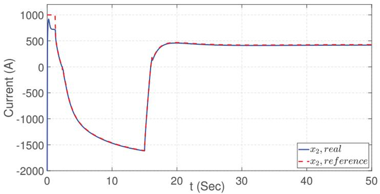
Figure 8. AES current control during regenerative braking.
