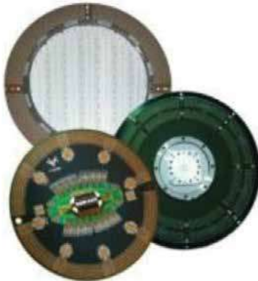
Figure 2. Cantilever, standard vertical and MEMS type probe cards.
