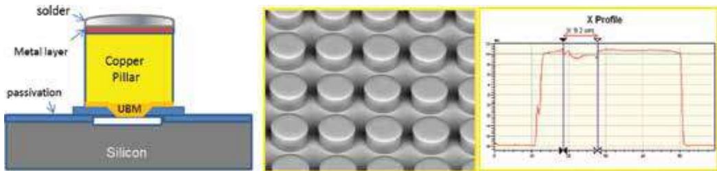
Figure 14. Images of copper pillars and lead-free micro-bumps at 50 \mu\text{m} pitch. The profile shows the pillar bump after probing with vertical MEMS probe technology.
