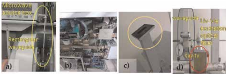
Figure 13. Common rectangular X-band waveguides and cavities and microwave source box used in laboratory. (a) typically the microwaves are combined with static \mathbf{H} fields Electromagnets are part of these equipments, (b) the inside of a microwave source box that delivers in a precise fashion microwaves from a few microwatts up to 180 mW, (c) view of the open end of a waveguide built with a flange to connect with other waveguides, and (d) a waveguide terminated in a rectangular TE_{011} cavity which is also fed with UV-Vis light through an optical fiber.
