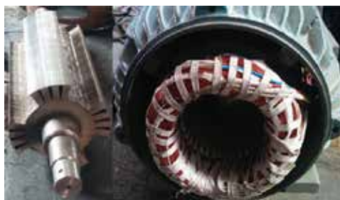
Figure 11. Fabrication details of 6-4-2 BDFRM.
