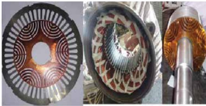
Figure 12. Fabrication details of 8-6-4 BDFRM.
