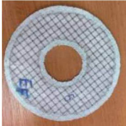
Figure 3. Woven fabric with inserted silver yarns in warp and weft.
