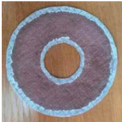
Figure 4. Same woven fabric with plasma copper coating.
