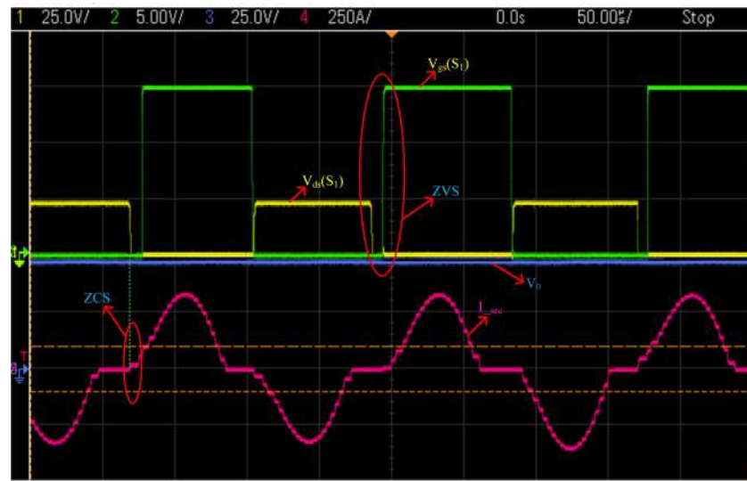
Figure 11. Experimental waveforms of the V_{gs} and V_{ds} showing ZVS operation under the worst condition.
