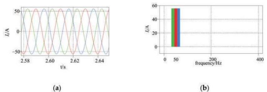
**Figure 7.** (a) Current curve of a GFM converter ( $P_{\text{set}} = 25,000$  W, SCR = 4.84); (b) current THD of a GFM converter ( $P_{\text{set}} = 25,000$  W, SCR = 4.84). (Green for phase A, red for phase B, blue for phase C).
