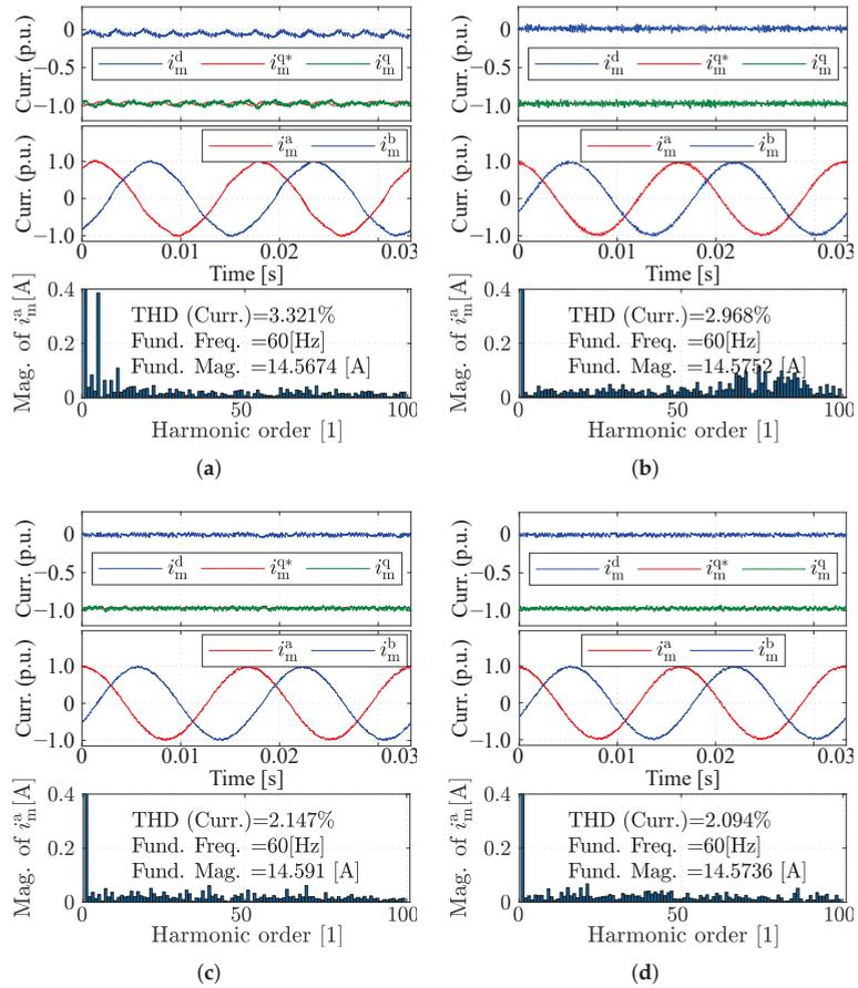
**Figure 5.** Generator side: (a) Classical DMPC (50%  $L_s$ ); (b) Classical DMPC (200%  $L_s$ ); (c) Classical DMPC (100%  $L_s$ ); (d) Proposed MIPC. For all sub-figures, from top to bottom are the dq-axis stator current and their references (base value 15 [A]), phase currents, and the current spectrum, respectively.
