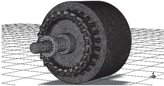
**Figure 8.** Meshing results of the DSOF motor.
