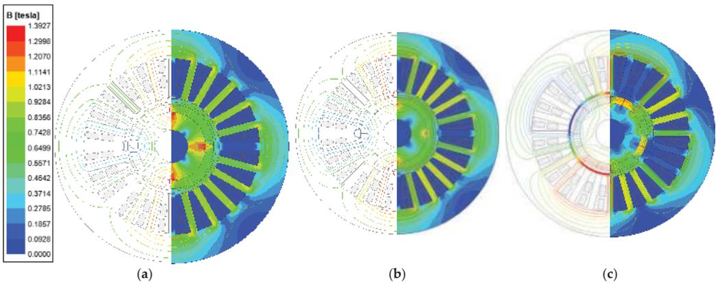
**Figure 8.** Magnetic flux density and lines distributions of HSPMMs with different magnetization methods under no-load condition. (a) Radial magnetization; (b) parallel magnetization; (c) Halbach magnetization.
