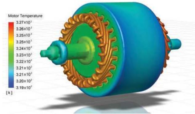
Figure 9. DSOF motor temperature distribution.
