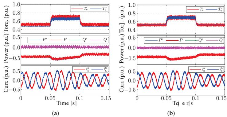
**Figure 7.** The control performance in the face of multiple mismatches: (a) Classical DMPC; (b) Proposed MIPC. For all sub-figures, from top to bottom are the generator torque (base value 30 [Nm]), the active and reactive power (base value 3475 [W]) and their references, and the phase currents on the grid side (base value 15 [A]), respectively.
