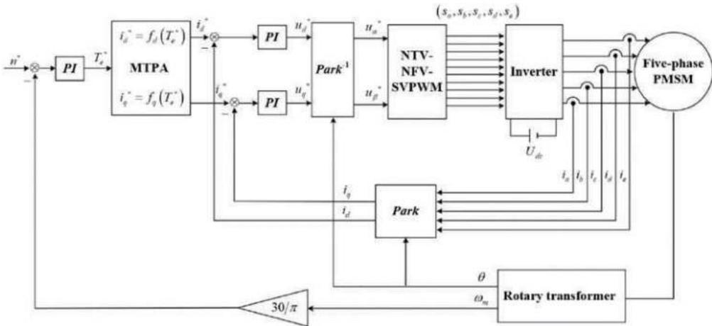
**Figure 19.** MPTA control of the five-phase PMSM block diagram.
