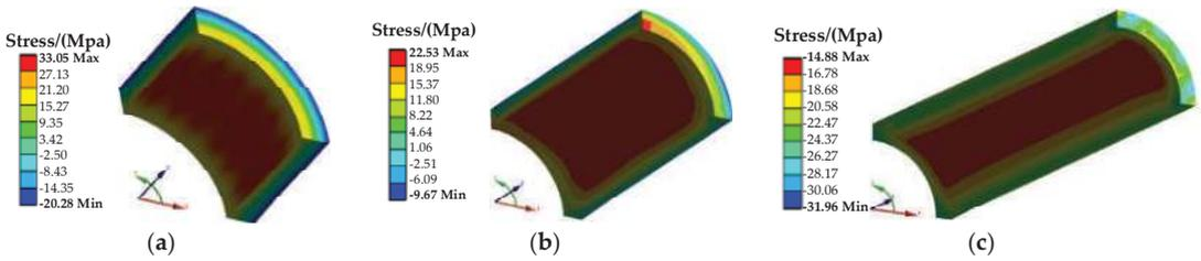
**Figure 20.** Permanent magnets radial stress distribution under the three cases at rated speed at a cold state: (a) Case 1; (b) Case 2; (c) Case 3.
