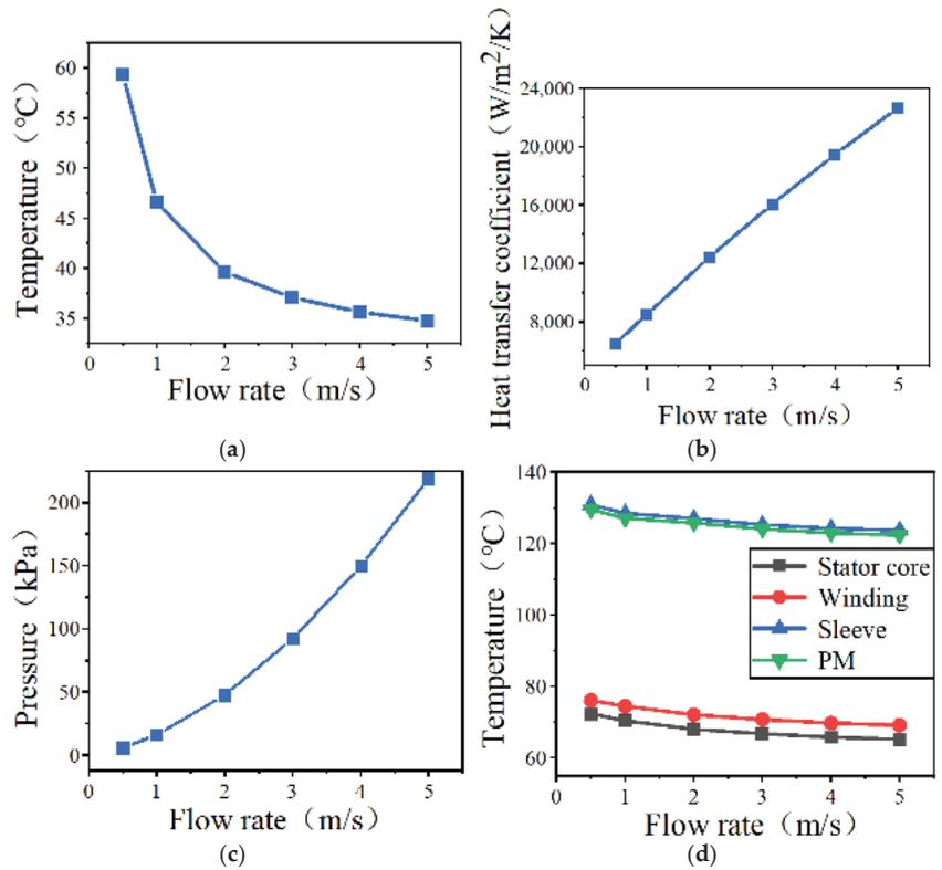
**Figure 16.** Thermal analysis results of HSPMMs at different cooling water flow rates. (a) Cooling water maximum temperature; (b) heat transfer coefficient; (c) inlet pressure; (d) motor maximum temperature.
