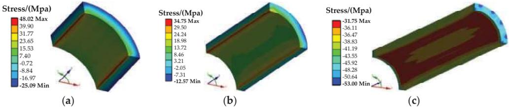
**Figure 23.** Permanent magnets’ radial stress distribution under the three cases at rated speed at a hot state: (a) Case 1; (b) Case 2; (c) Case 3.
