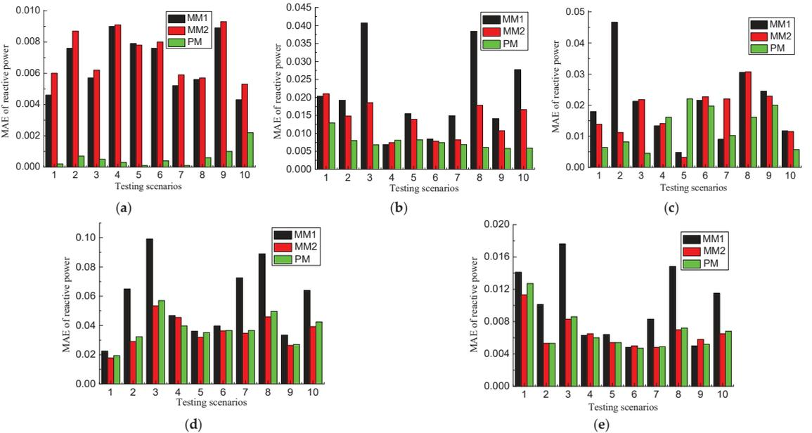
**Figure 6.** Reactive power response error of three equivalent models. (a) Pre-fault phase. (b) Early fault phase. (c) Quasi-steady-state phase during the fault. (d) Early fault recovery phase. (e) Quasi-steady-state phase during the fault recovery.
