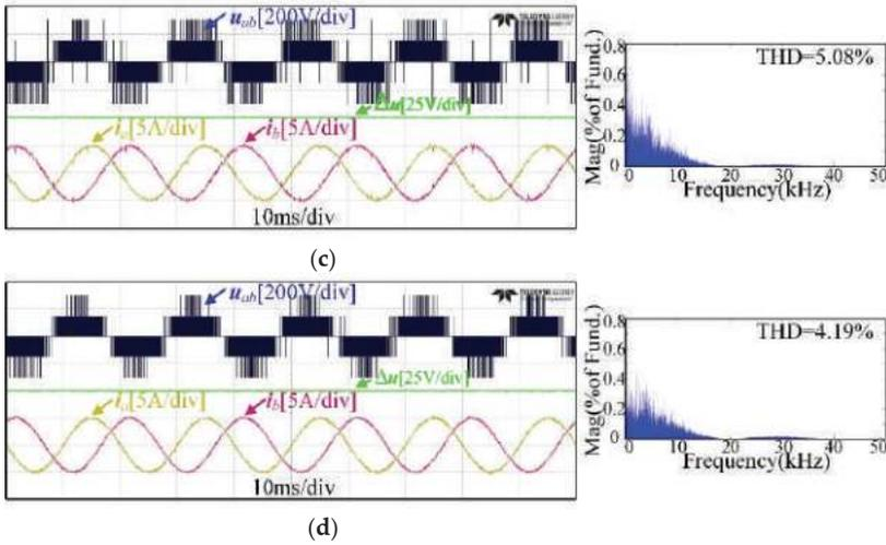
**Figure 9.** Experimental waveform comparisons ( $i_{ref} = 5A$ ). (a) Waveforms under the conventional MPC scheme. (b) Waveforms under the conventional MFPC scheme in [20]. (c) Waveforms under the conventional MFPC scheme in [30]. (d) Waveforms under the proposed MFPC scheme.
