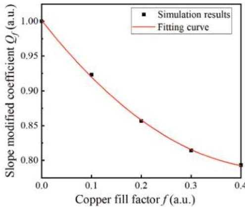
Figure 6. Slope-modified coefficient versus copper fill factor.
