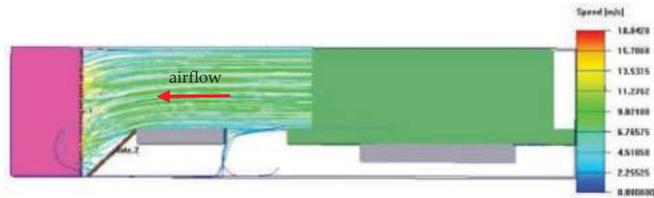
Figure 7. Airflow speed vector results before optimization.
