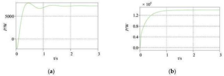
**Figure 13.** (a) Active power of the GFL converter ( $P_{set} = 7000$  W, SCR = 4.84); (b) active power of the GFL converter ( $P_{set} = 140,000$  W, SCR = 4.84).
