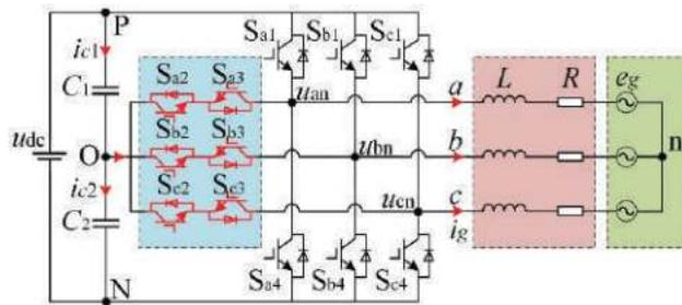
Figure 1. Topology of the T-type three-level grid-tied inverter.
