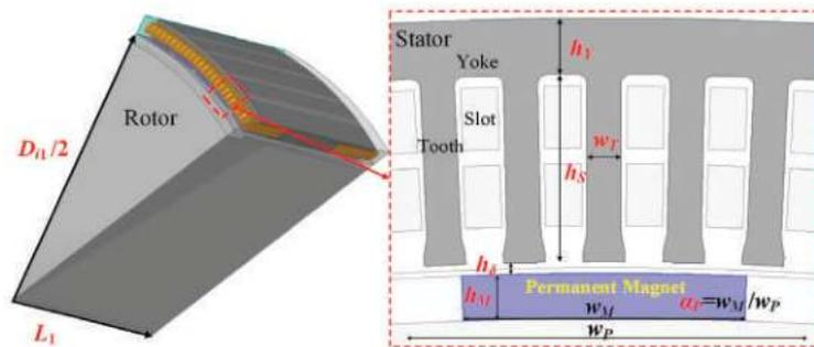
**Figure 7.** Generator structure and its design parameters.
