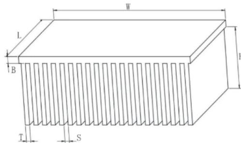
**Figure 1.** Structural diagram of the forced-air-cooled heat sink.
