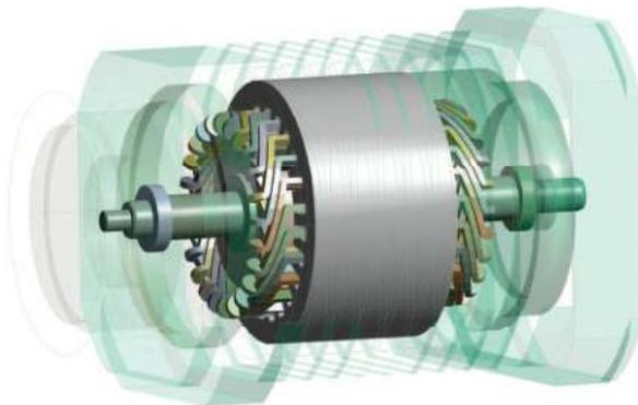
**Figure 7.** 3D CFD model of the DSOF motor.
