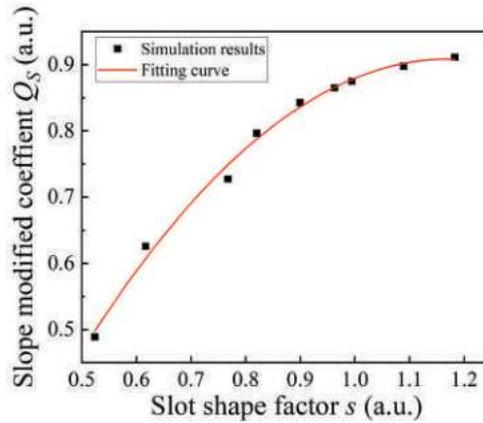
Figure 4. Slope-modified coefficient versus slot shape factor.
