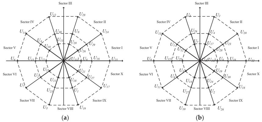
**Figure 18.** Space voltage vector distribution in the fundamental and third harmonic coordinate system. (a) Fundamental  $\alpha_1-\beta_1$  coordinate system vector distribution. (b) third harmonic  $\alpha_3-\beta_3$  coordinate system vector distribution.
