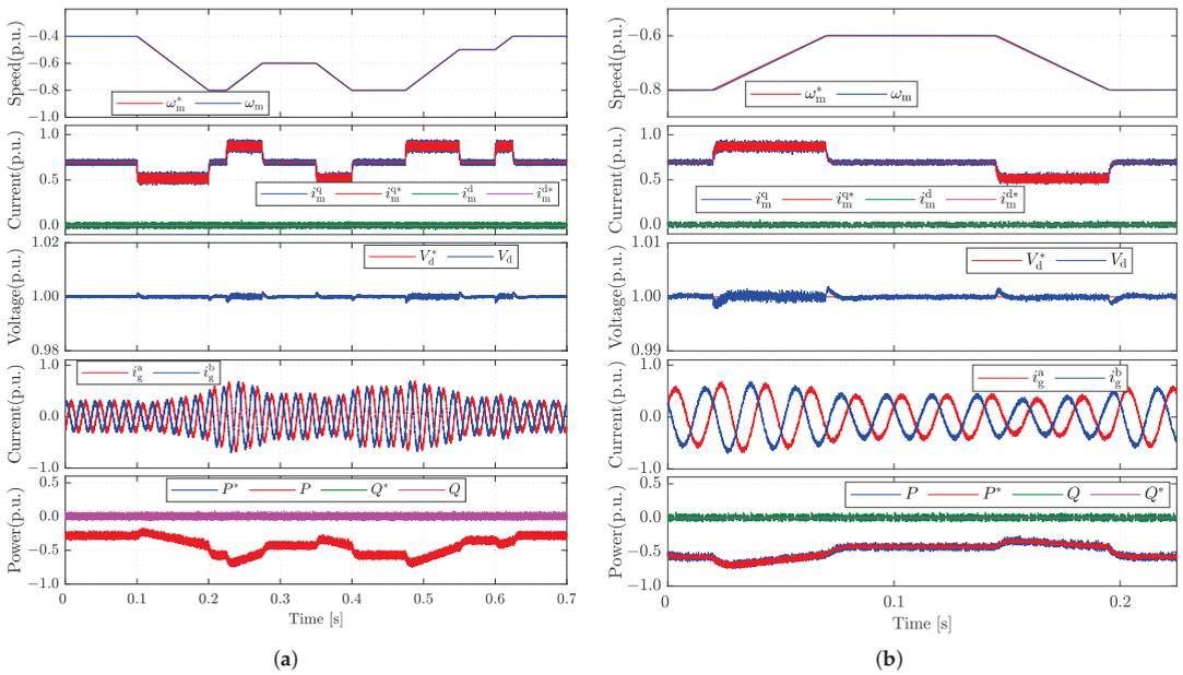
**Figure 3.** Performance of the proposed MIPC method. (a) Overall control performance. (b) Zoomed control performance. From top to bottom are the PMSG mechanical speed, stator dq-axis currents, DC-link voltage, grid-side currents, active and reactive power, and their references, respectively. The speed base is 125 r/min. The current base is 15 A.
