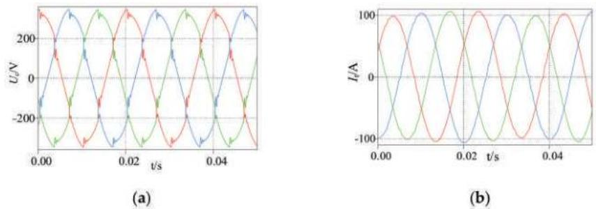
**Figure 15.** (a) Voltage of the GFM converter ( $P_{set} = 140,000$  W, SCR = 29.04); (b) current of the GFL converter ( $P_{set} = 22,000$  W, SCR = 4.84). (Green for phase A, red for phase B, blue for phase C).
