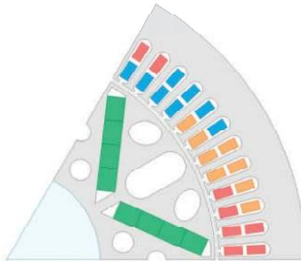
Figure 7. The FEM of IPMSM.
