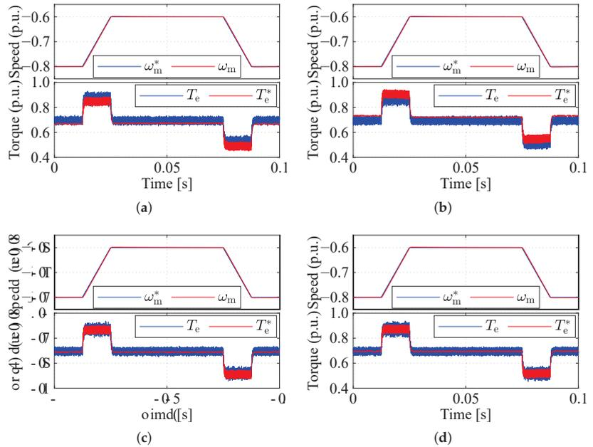
**Figure 4.** Performances under permanent-magnet flux linkage variations: (a) Classical DMPC (50%  $\psi_{pm}$ ); (b) Classical DMPC (200%  $\psi_{pm}$ ); (c) Classical DMPC (100%  $\psi_{pm}$ ); (d) Proposed MIPC. For all sub-figures, from top to bottom are the generator speed (base value 125 [rad/s]) and the generator torque (base value 29 [N · m]), respectively.
