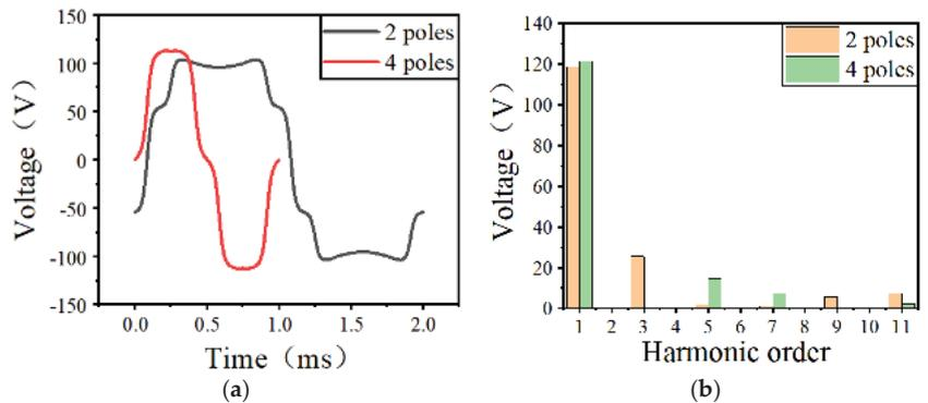
**Figure 1.** Waveforms and FFT analysis results of back EMF for 2 poles and 4 poles HSPMMs. (a) Waveforms; (b) FFT analysis results.
