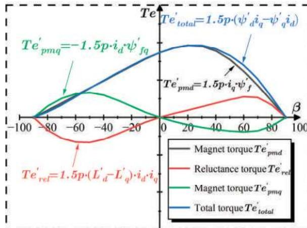
Figure 4. Relationships between each torque and current angle.
