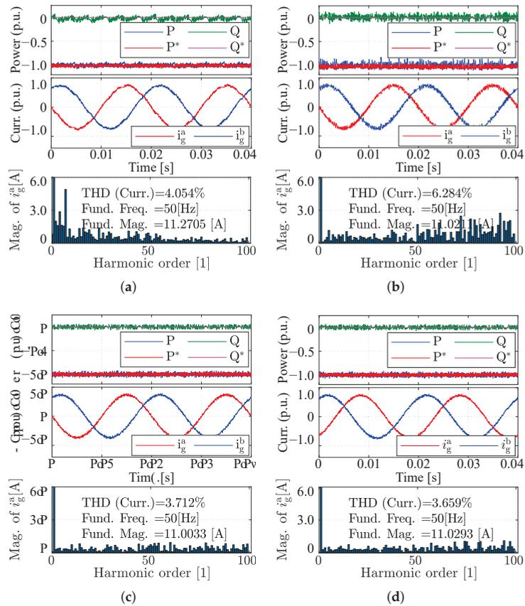
**Figure 6.** Grid side: (a) Classical DMPC (50%  $L_g$ ); (b) Classical DMPC (200%  $L_g$ ); (c) Classical DMPC (100%  $L_g$ ); (d) Proposed MIPC. For all sub-figures, from top to bottom are the active and reactive power (base value 3475 [W]) and their references, phase currents, and the current spectrum (base value 15 [A]), respectively.
