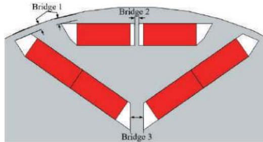
**Figure 9.** Rotor magnetic bridge schematic diagram.
