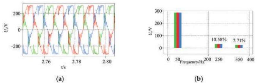
Figure 12. (a) Voltage of a GFM converter ( $P_{set} = 140,000$  W, SCR = 29.04); (b) THD of a GFM converter ( $P_{set} = 140,000$  W, SCR = 29.04). (Green for phase A, red for phase B, blue for phase C).
