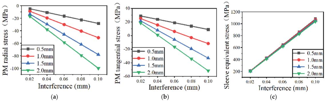
**Figure 20.** The maximum stress of the rotor variations with sleeve thickness and interference. (a) PM maximum radial stress; (b) PM maximum tangential stress; (c) sleeve maximum equivalent stress.
