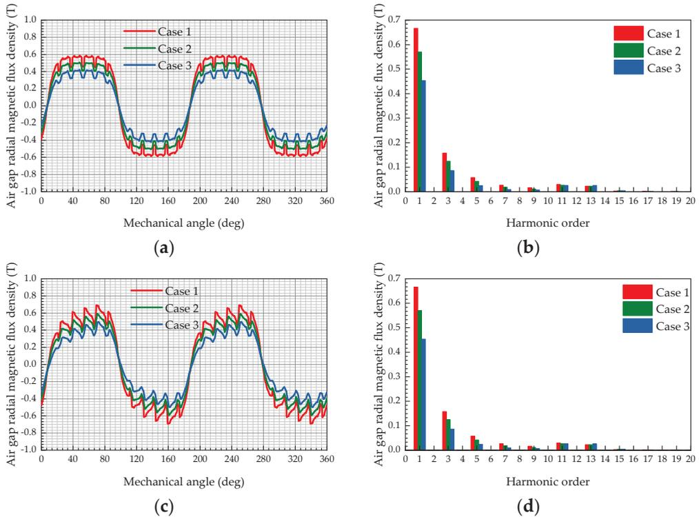
**Figure 13.** Radial air-gap flux density and Fourier transforms under three cases at no load and rated load: (a) radial air-gap flux density at no load; (b) Fourier transforms results at no load; (c) radial air-gap flux density at rated load; (d) Fourier transforms results at rated load.
