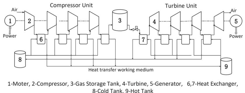
**Figure 1.** Advanced adiabatic compressed-air energy storage system.
