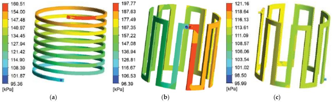
**Figure 14.** Pressure distribution of the three cooling channel structures. (a) Spiral structure; (b) axial structure 1; (c) axial structure 2.
