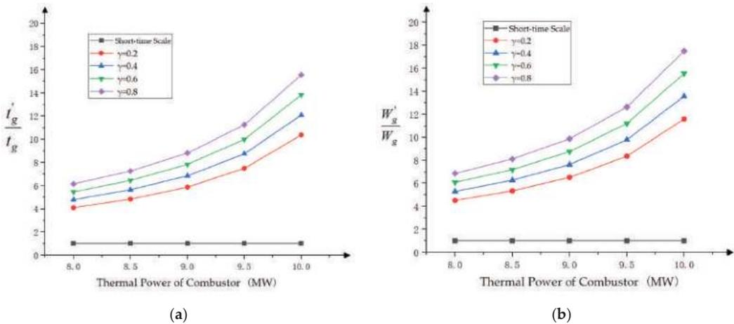
**Figure 6.** Relation diagram of different injection coefficients and burner thermal power with power-generation capacity and power-generation time: (a) power-generation time and (b) power-generation capacity.
