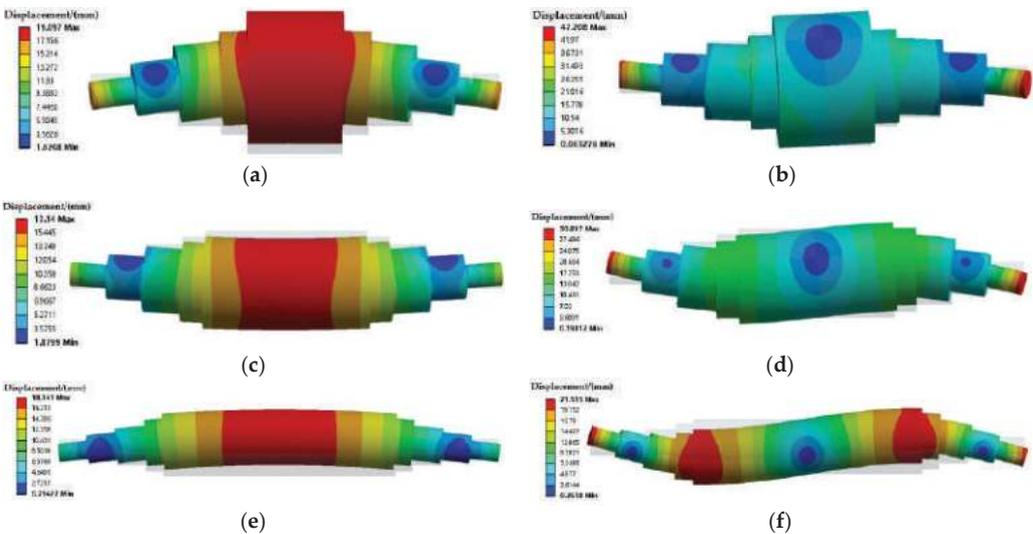
**Figure 24.** Rotor dynamic characteristics under the three cases: (a) first-order mode for Case 1; (b) second-order mode for Case 1; (c) first-order mode for Case 2; (d) second-order mode for Case 2; (e) first-order mode for Case 3; (f) second-order mode for Case 3.
