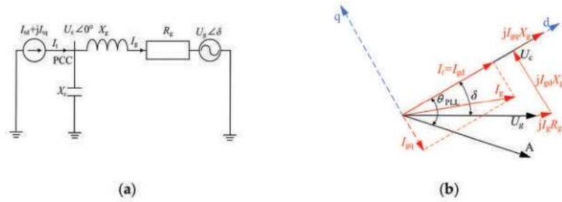
**Figure 4.** (a) Equivalent circuit diagram of a GFL converter; (b) phasor diagram of GFL converter.
