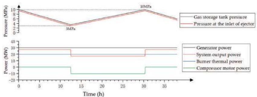
Figure 7. Operating parameters under continuous-output conditions.
