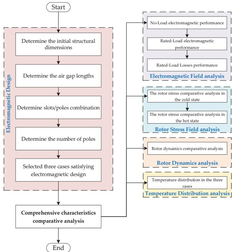
**Figure 1.** Comprehensive characteristics comparative analysis and design process.
