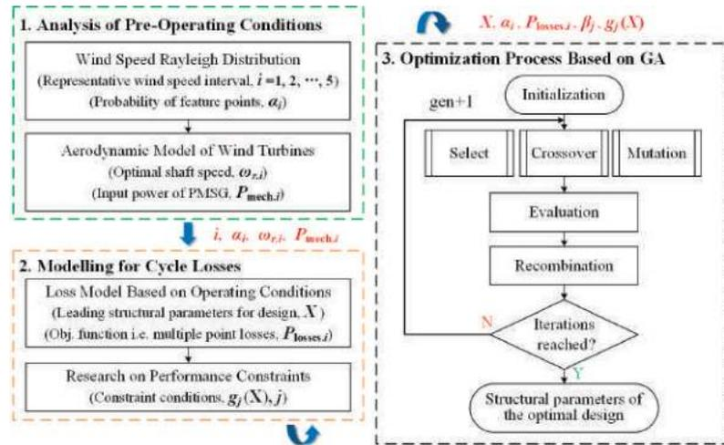
Figure 5. Flowchart of cycle efficiency design optimization.
