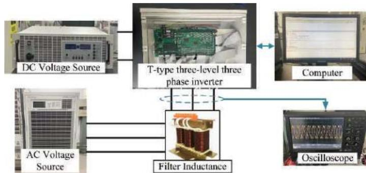
Figure 7. T-type three-level three-phase grid-connected inverter experimental platform.
