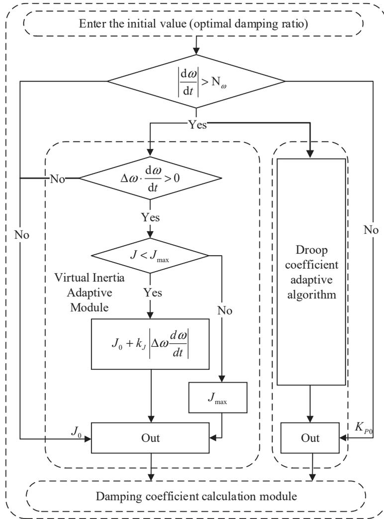
Figure 6. Core algorithm flow chart.
