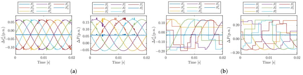
Figure 9. Estimated d-axis current variation and active power variation caused by different voltage vectors using (a) the proposed MIPC and (b) classical MIPC [24].  $S_x^1-S_x^8$  denote the available voltage vectors of the machine side ( $x = m$ ) and the grid side ( $x = g$ ), respectively.
