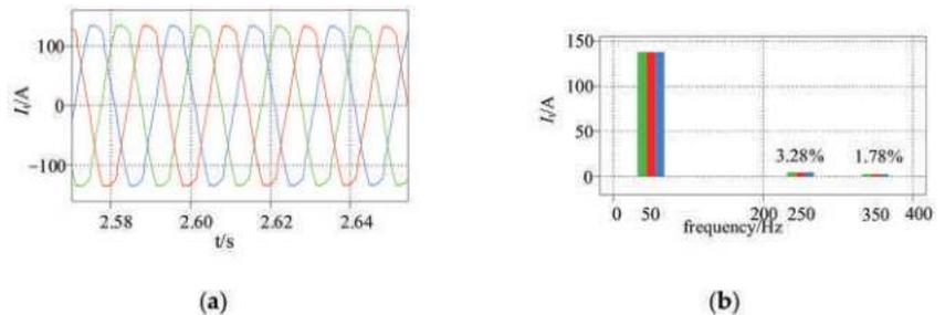
**Figure 10.** (a) Current of a GFL converter ( $P_{set} = 25,000$  W, SCR = 4.84); (b) current THD of a GFL converter ( $P_{set} = 25,000$  W, SCR = 4.84). (Green for phase A, red for phase B, blue for phase C).
