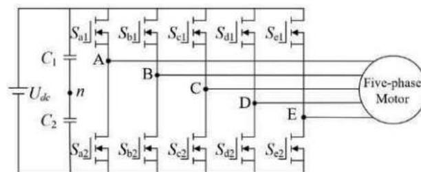
Figure 17. The topology of the five-phase half-bridge inverter.
