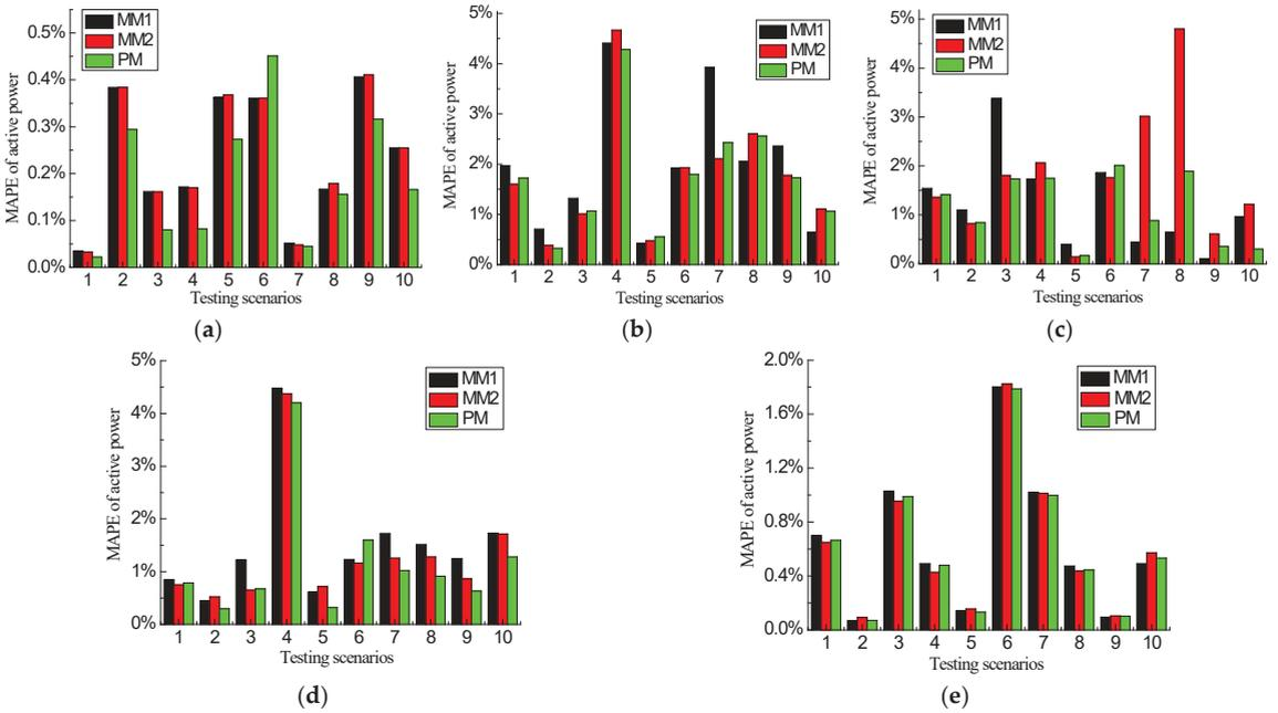
**Figure 5.** Active power response error of three equivalent models. (a) Pre-fault phase. (b) Early fault phase. (c) Quasi-steady-state phase during the fault. (d) Early fault recovery phase. (e) Quasi-steady-state phase during the fault recovery.
