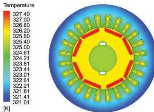
Figure 10. DSOF motor cross-section temperature field contour.
