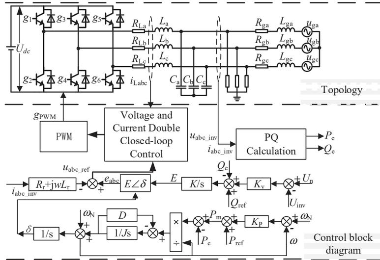
Figure 1. Topology and control block diagram of VSG.
