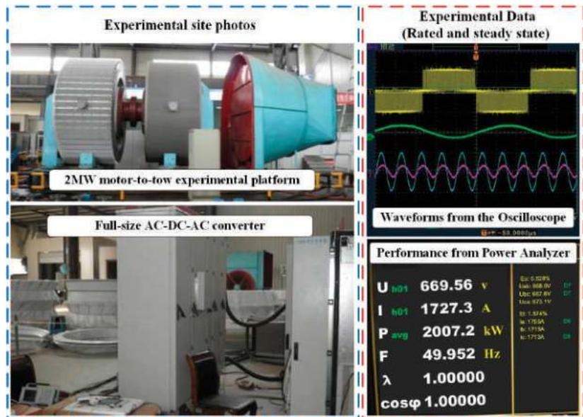
Figure 9. Experimental site photos and performance demonstration.
