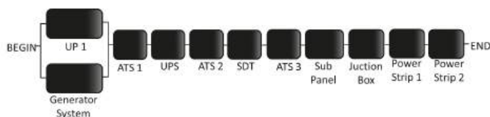
Figure 12. RBD model of the Tier I power infrastructure.
