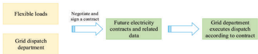
Figure 4. Real-time dispatching process of power grid considering flexible load.
