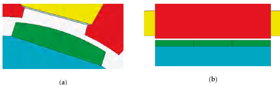
Figure 5. Magnet segmentation: (a) Segmentation A, parallel to the axis (two magnets per pole); (b) Segmentation B, parallel to the circumference (three magnets per pole).
