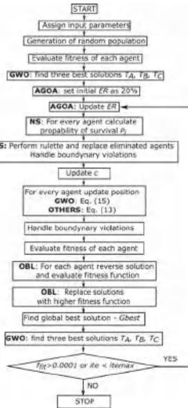
Figure 5. Flow chart of the GOA algorithm with proposed modification.
