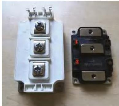
**Figure 5.** The 1.2 kV SiC MOSFET power module, part no. CAS120M12BM2, used in the project, with a rated current of 138 A (left) and a 36% smaller 1.2 kV SiC MOSFET power module, part no. CAB450M12XM3, with a rated current of 409A, available on the market from mid-2019.
