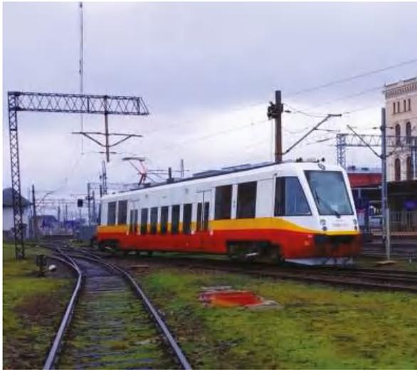
**Figure 2.** The EN81 series 3 kV DC electric passenger railcar used for the field trial with the roof-mounted SiC-based DC power electronic traction transformer (PETT) prototype.
