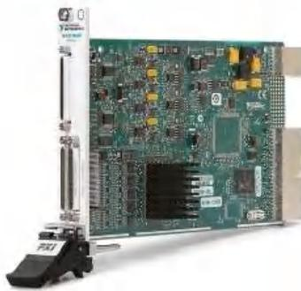
Figure 1. Field-Programmable Gate Array (FPGA) PXI-7854R illustration [11].
