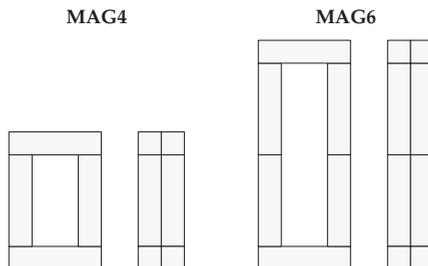
**Figure A2.** Single-phase multi air gap MFT core assembly: MFT4 with 4 air gaps (left) and MFT6 with 6 air gaps (right).
