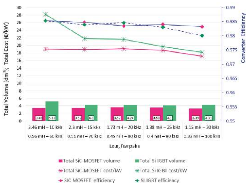
Figure 13. Efficiency, cost and total volume comparison of the two converters at 75 A output current and 50 °C heat sink temperature.
