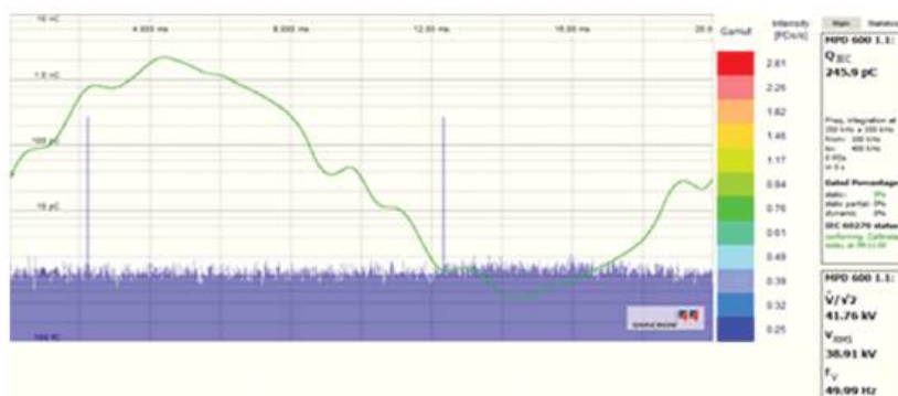
Figure 1. Test voltage waveform and the partial discharge (PD) pattern during the high-voltage (HV) test.
