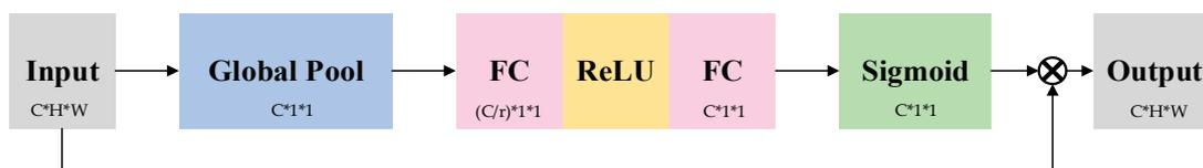
Figure 3. SENet attention structure diagram.
