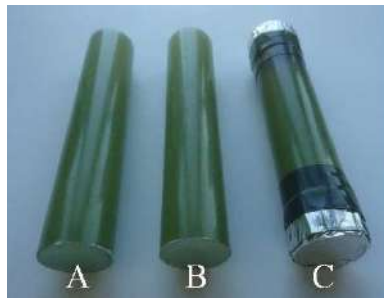
Figure 2. Glass-reinforced epoxy (GRE) material samples of the high voltage alternating current (HVAC) composite insulator carrying rod. From the left: reference sample—group A; thermally aged sample—group B; and DC and thermally aged sample—group C, with visible electrodes attached to the sample's front surfaces.
