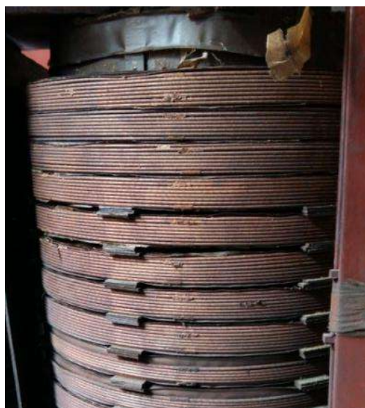
Figure 5. Example of deformation introduced into windings of a transformer: compression (reduced inter-disc distances in three gaps)—Def. 3.
