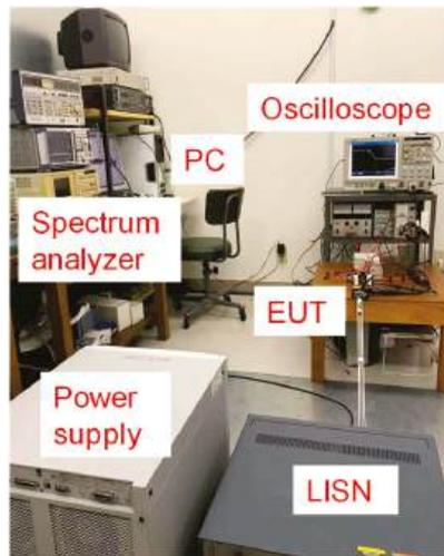
**Figure 5.** The experimental setup of conducted noise measurement.
