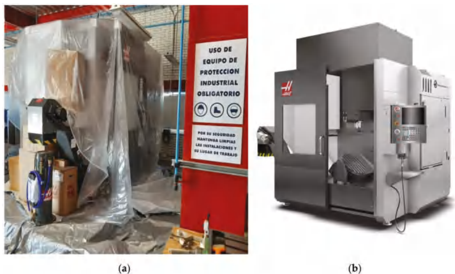
Figure 1. Computer Numerical Control (CNC): (a) CNC installed at the Orthotics and Prosthetics Laboratory (OPL); (b) CNC Haas Automation model UMC-750.
