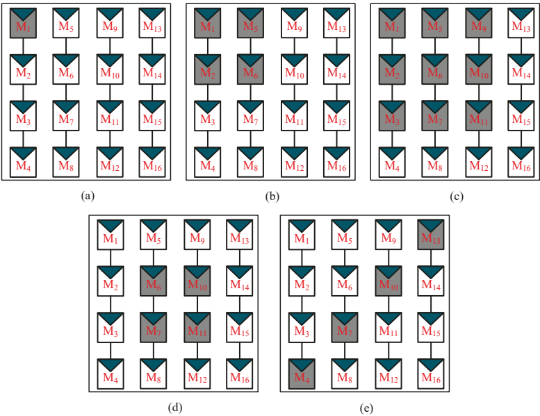
Figure 7. Shading pattern designs for PV array configuration schemes: (a) one module, (b) short wide, (c) long narrow, (d) central, and (e) diagonal.
