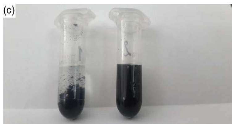
Figure 3. SEM morphological details of CNTs as received from the manufacturer, before (a) and after (b) loading with the mixture CHX/AgNPs (High magnification, 100,000 \times ); (c) photographic image of colloidal CNTs in distilled water (left) compared to colloidal mixture CHX/AgNPs (right).
