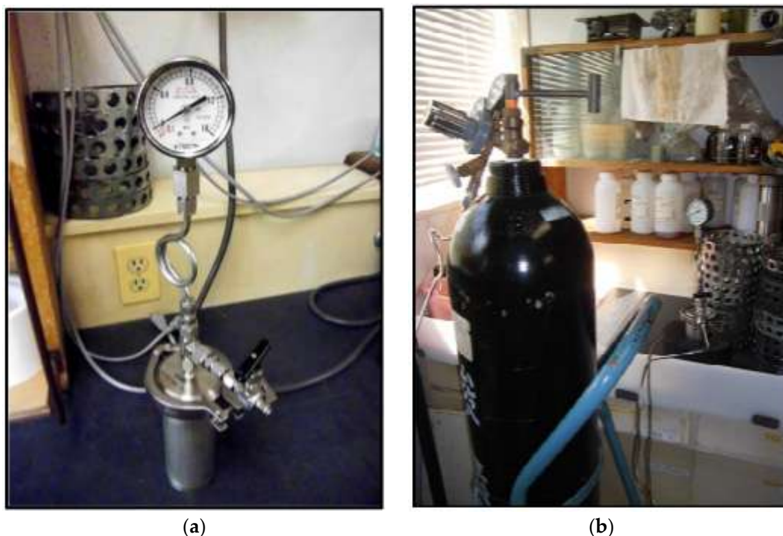
Figure A3. Charge oxygen gas under 0.35–0.50 MPa at room temperature.
