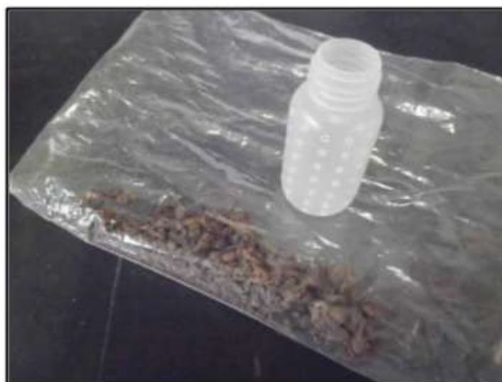
Figure A1. Put pulp in polyethylene plastic bag and make pulp into small particles (diameter 5–10 mm).
