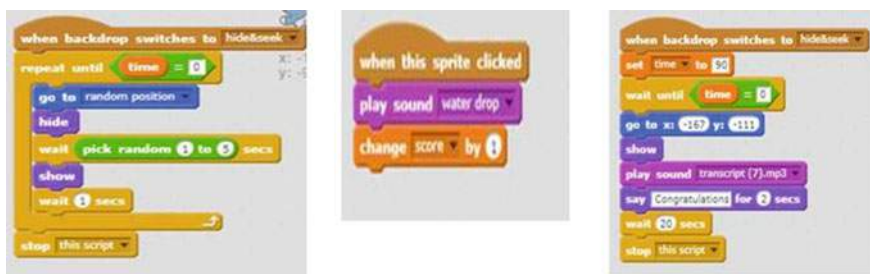
Fig. 11.8 Hide-and-seek code (object-orientation, decomposition, variables, behavior, values)
