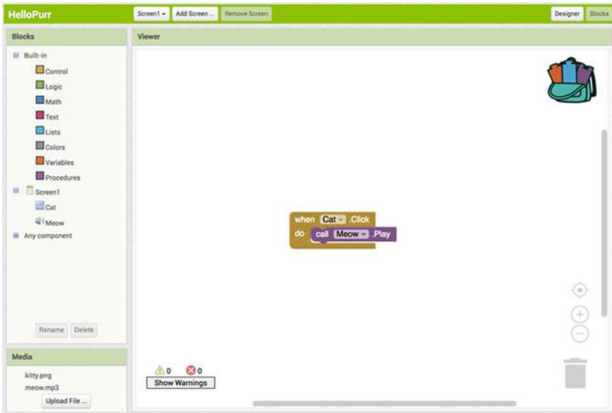
Fig. 3.2 App Inventor’s blocks editor. Blocks code is typically read left to right, top to bottom. In this example, one would read “when Cat click, do call Meow play,” that is, play the meow sound when the cat is clicked
