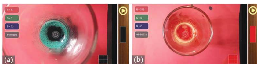
Figure 8. Image of the chemical reaction performed and record of the R -index using ColorMeter Free app. (a) Addition of blue food dye at the beginning of the reaction. (b) View of the system once the reaction was completed.
