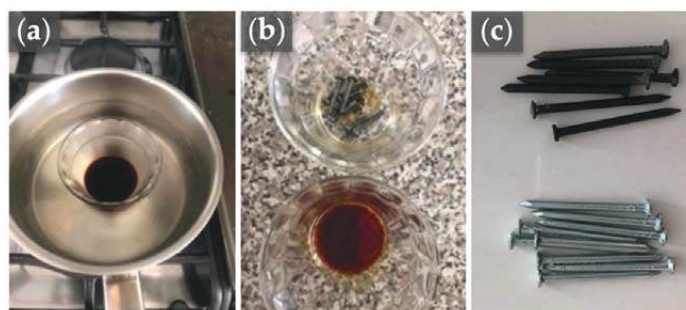
Figure 5. (a) Heating the mixture of nails and iodine tincture in a water bath. (b) Separation of the iodine tincture and nails after the reaction. (c) Comparison of the nails before and after the oxidation reaction (Images extracted from a students' report).
