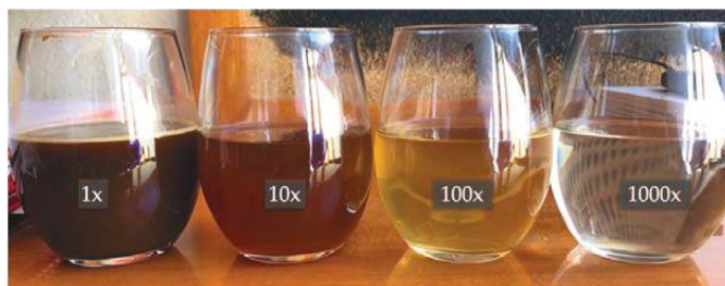
Figure 4. Sucrose solutions diluted 1000 times using coffee as colorant (Image extracted from a students' report).
