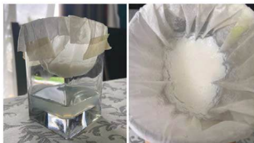
Figure 7. Filtration of casein precipitated from a sample of milk (Images extracted from a students' report).
