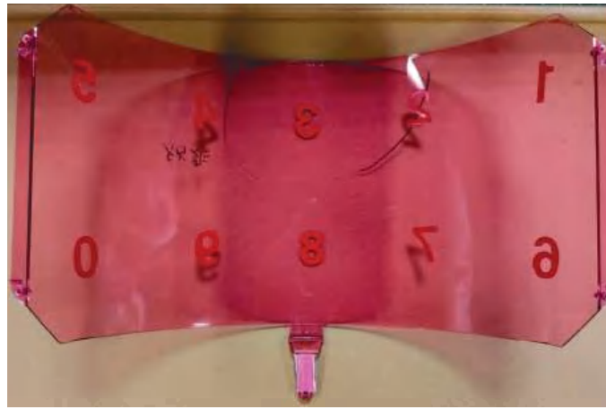
Figure 5. The ski goggles' lens sample. It is wide and curved; thus, we mark its surface to be easily controlled by cameras.
