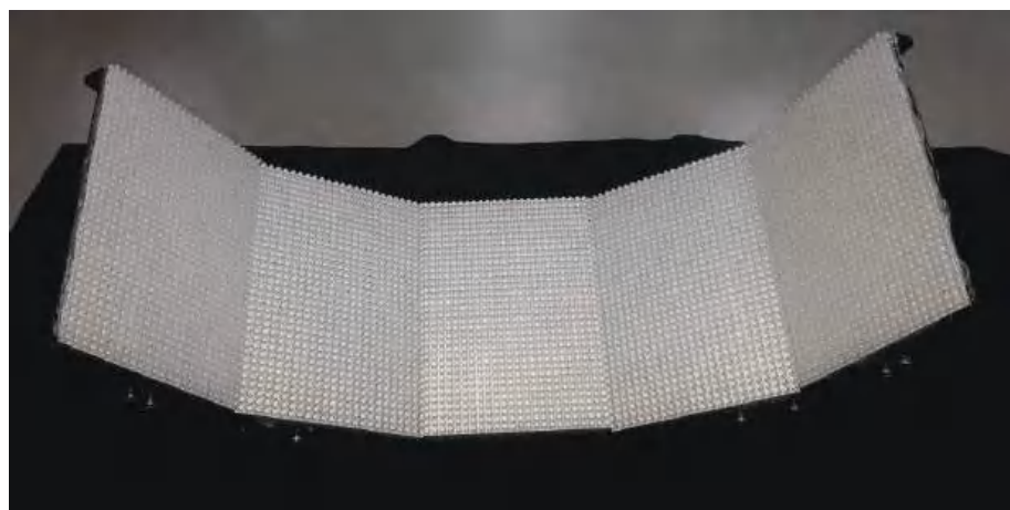
Figure 6. The most that a custom light source meets the curvature of the ski goggles lens. Five dot matrix LED modules are connected by an angle of 125°.
