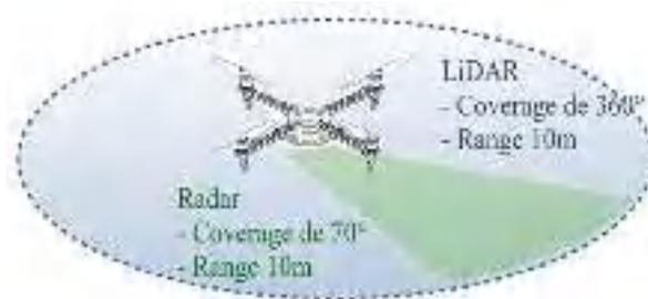
**Figure 5.** LiDAR and Radar sensor range.
