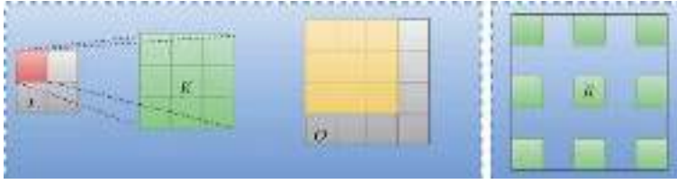
Figure 3. Left: A demonstration of transposed 2D convolution with a 3 \times 3 \times D_I kernel (stride = 1, padding = 0), I \in \mathbb{R}^{2 \times 2 \times D_I} is the spacial input and O \in \mathbb{R}^{4 \times 4} is the 1-channel output feature map. Note that the receptive fields in O can overlap and we normally sum the values where output overlaps. Right: A dilated kernel for increasing the receptive fields in the input, where the empty space between each element represents 0.
